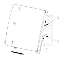
Removal: Insert the screwdriver into E, pull down the snap and make it tilt outward in the meantime, then it can be removed from the rail.
